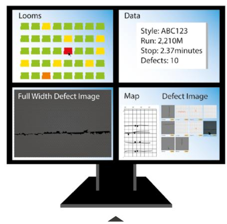
In addition to very sensitive detection from powerful defect detection algorithms the FFI systems can be set up with real time defect classification and grading, so that auto stopping for certain defects and not others can be implemented and reports can be run from the system data, without pre analysis by an operator.
